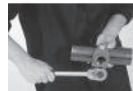
Check the pipe surface. The hole must be cut or drilled on centerline of pipe and in dimensions conform QUIKCOUP® specifications.
